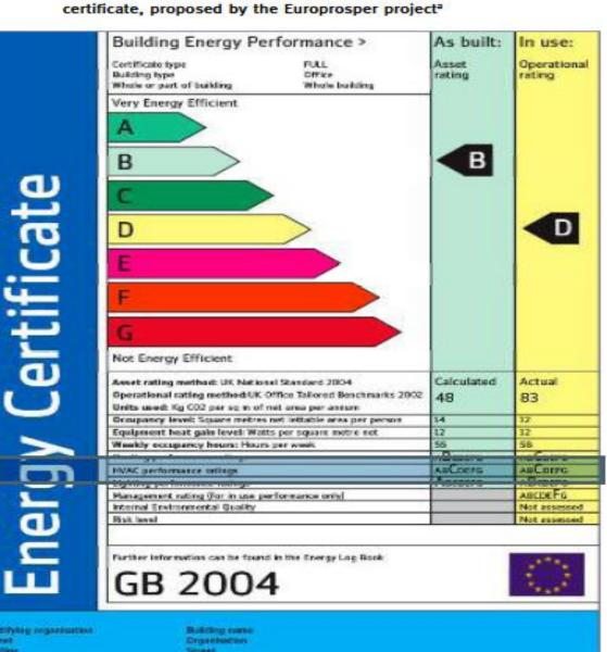
Figure V. Illustration of a possible format for a non-domestic building energy
