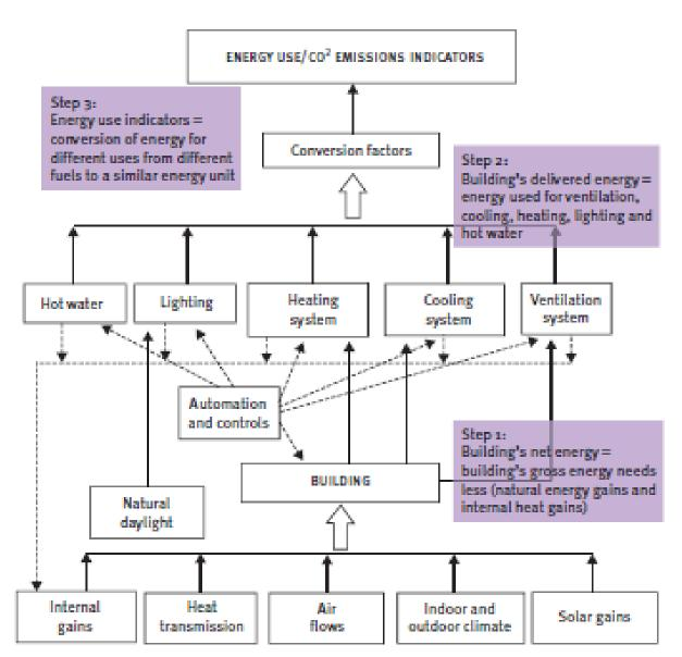
The calculation of energy use in buildings is based on the characteristics of the building and its installed equipment. It is structured in three levels as illustrated below and the calculation is performed from the bottom up.
