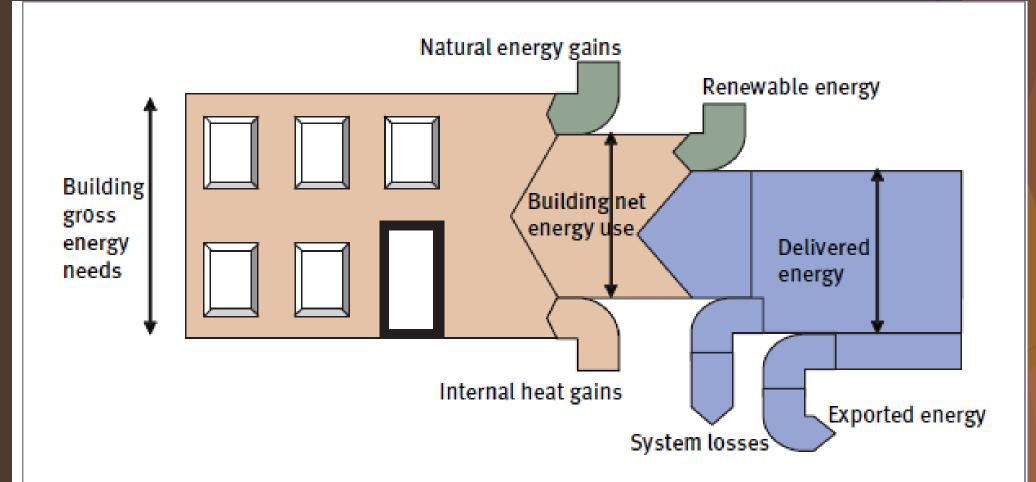
Figure above illustrates the typical energy flows in a building. The building gross energy needs represent the anticipated buildings requirements for heating, lighting, cooling, ventilation, air conditioning and humidification.
